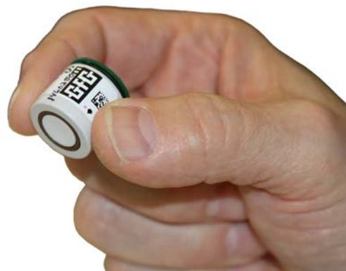
**Larger sized sensors have more room for internal filters. The larger size of the sensing electrode and greater volume of electrolyte make them harder to destabilize as well.**
