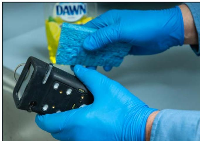
**Use mild dish soap to clean the instrument, and a damp sponge to wipe it off with fresh water. Try not to get soapy water into the sensor openings or audible alarm.**
