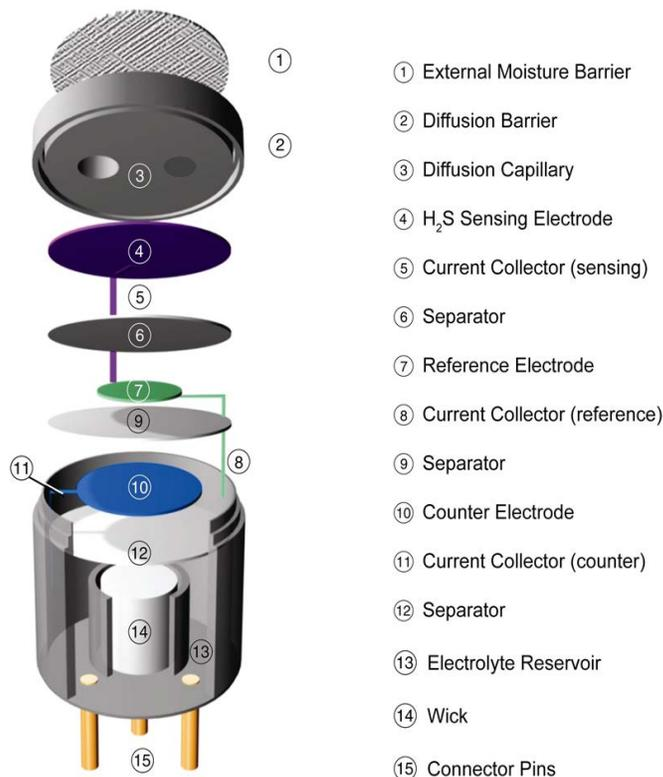
**Electrochemical sensors used to measure CO and other toxic gasses are complicated devices with many internal components. CO sensors often include filters to protect the sensor from exposure to alcohol and other VOC vapors.**
