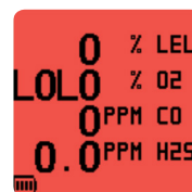
Red display in alarm conditions
